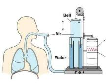
With this device we create a closed system between the lungs and the spirometer, so at any time the person inhales air from the cylinder of the device and exhales air back to the cylinder. In the way of expiration, the device is linked to another device which can adsorb all CO<sub>2</sub>, what remains in the spirometer is oxygen which is inhaled by the person and so on.
