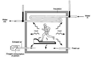
the water getting out, you don't have the same temperature, actually you have higher temperature. The difference in the temperature is the heat which is released from the body and gained by water. If you know the flow rate of water per time unit and you know the number of calories which is gained by water at the same time, you can calculate by a direct way the amount of heat which is produced by the body.
